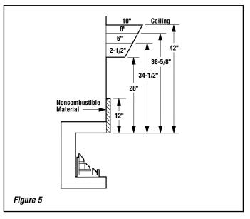
**Example:** The bottom of the mantel may project from the wall a maximum of 2-1/2" at a minimum of 8" above the opening. The top shelf of the mantel may project a maximum of 6" at a minimum of 14-1/2" above the opening.
